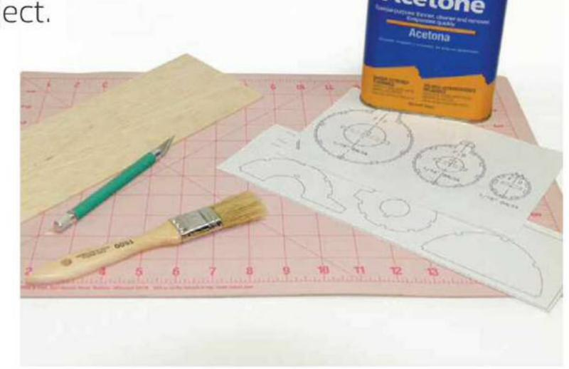
Here are the materials you need: photocopies of the parts templates, a cheap paintbrush, acetone, and balsa or plywood sheet stock. CAUTION: Acetone is a volatile solvent. Make sure your work area has adequate ventilation.
